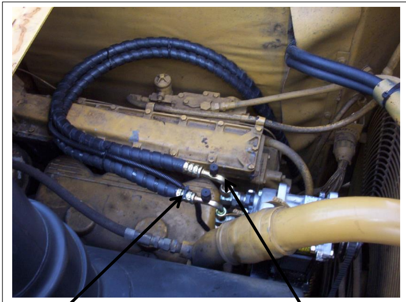
#8 hose to condenser
